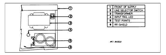
Figure C-3. Series 667xA Line Select Switch
